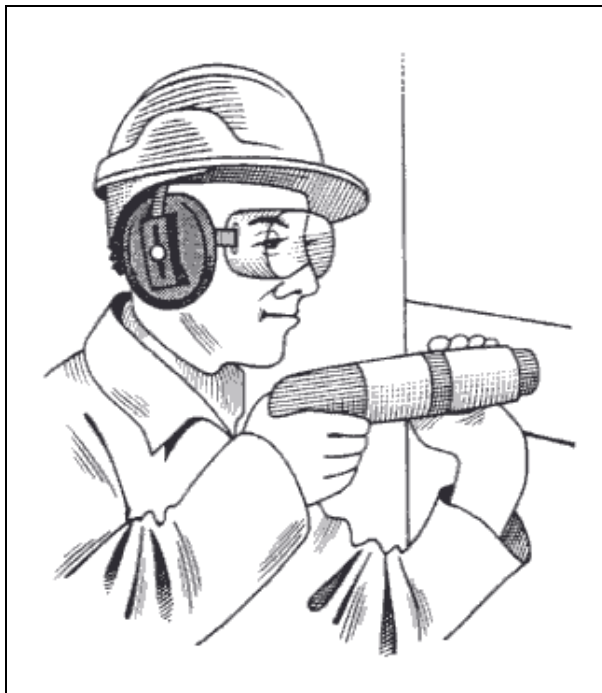
Figure 42. Use of hearing and eye protection by the operator of a cartridge gun, who is also wearing a helmet
